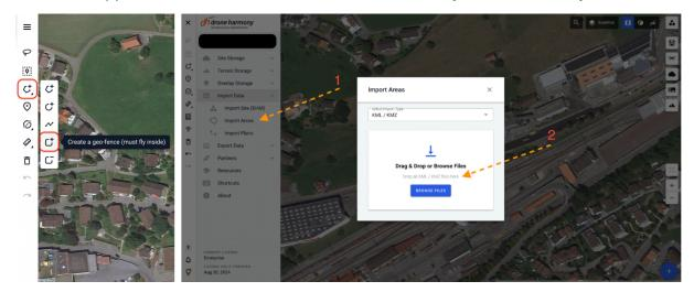
4. **Geo-Referenced 3D No-Fly Zones:** These can be provided via \*.kml files or by drawing within the app. No-fly zones are areas where the drone should not enter for safety or privacy reasons.
