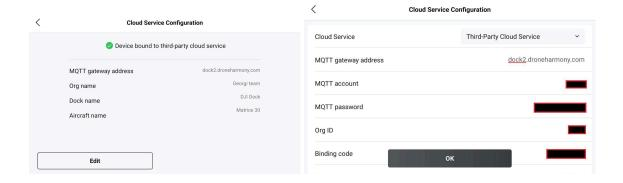
Next, you may verify the successful setup of the cloud service by checking the live feed(s) and telemetry of your dock(s) and drones in the Drone Harmony dock application:
