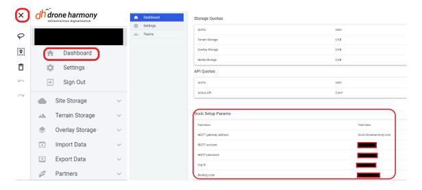
To set up the DJI dock's communication with the Drone Harmony Cloud Service, these presented parameters need to be copied into the DJI Cloud Service Configuration of the DJI Pilot 2 application, which runs on the DJI dock remote controller:
