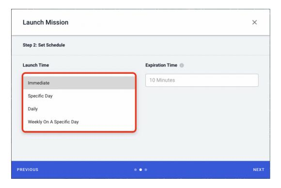
1. Immediate task - This will be executed immediately after you finish all launching steps. The task will expire in the timeframe that you have set in any option for scheduling including this one if it is not possible to complete the task for some reason such as weather conditions etc. (these tasks will appear in the history tab as failed)
