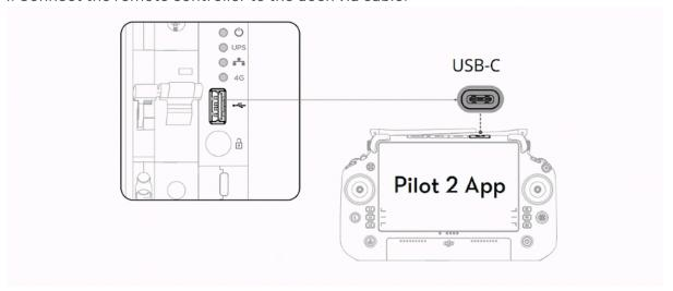
2. Run the DJI Pilot 2 app on your controller and tap open the dock cover. The dock will appear as a device in the same window that is used to represent aircraft.
